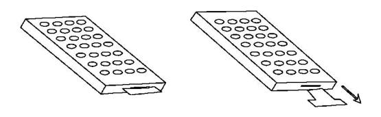
2.Before you using the remote controller, please remove the transparent plastic, which is designed to disconnect the battery
